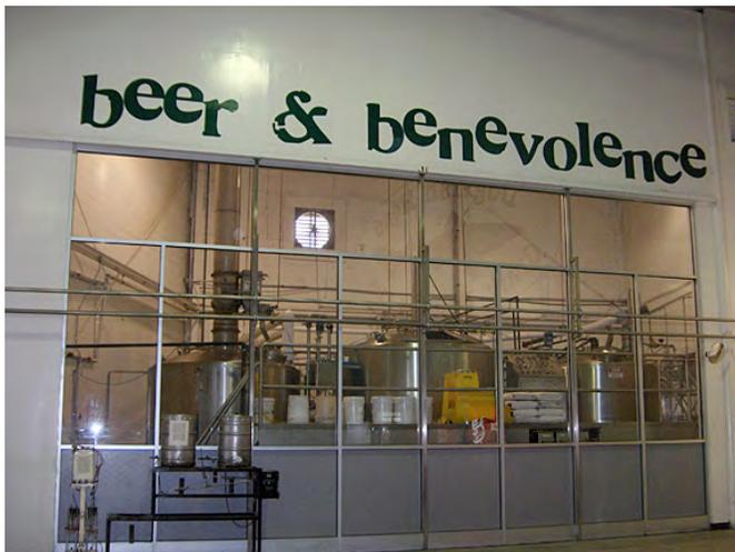
*The brew room. The 2 small converted kegs in front were the original brew set-up for the brewery. The original bottler is on the left. "Sir Hops Alot" can be seen next to the large pipe on the left. This device is used to release the hops every 60 seconds in the 60, 90, and 120 Minute IPAs.*
